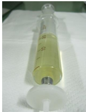
3. Attach the membrane filter (0.5µm) to the tip of a syringe.
