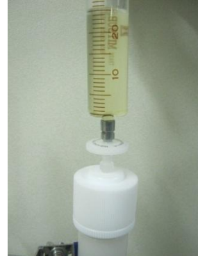
4. The sample is poured into CHIRALFLASH.
