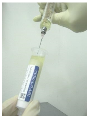
1. The sample solution is added to the injection cartridge.
