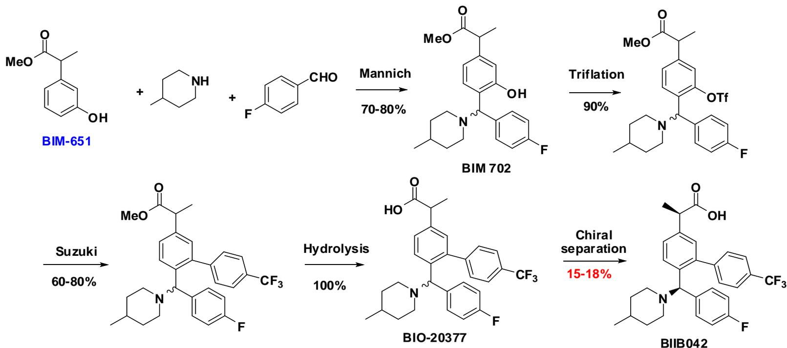
The Mannich reaction established the framework for **BIIB042** in the first step producing **BIM-702**, and chiral chromatography was employed to separate the four stereoisomers.
